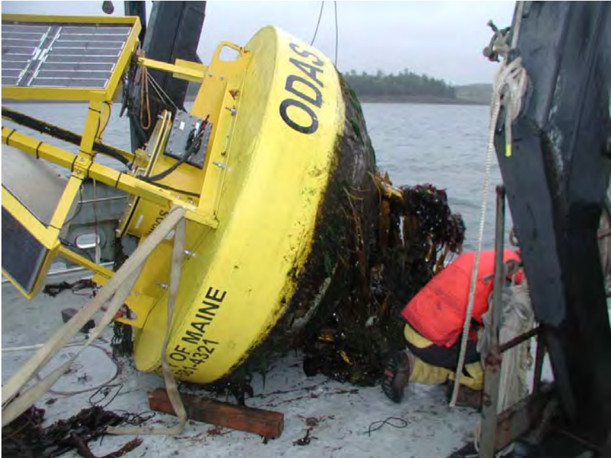
Figure 3-6: Buoy F01 early spring bio-fouling (April 2008)
