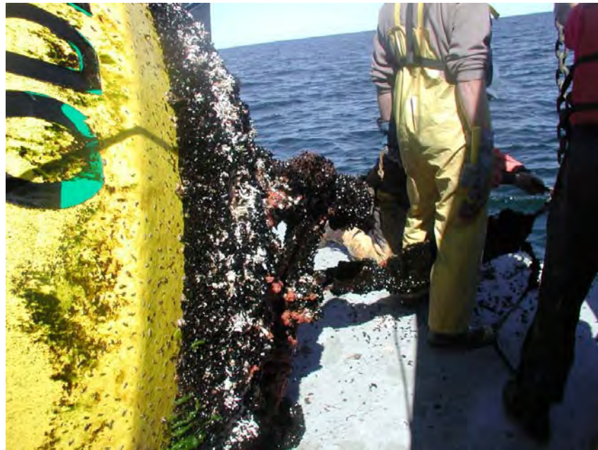
Figure 3-3: Buoy E01 summer bio-fouling (September 2006)
