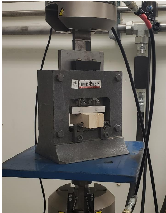
Figure 6. Block shear testing.
