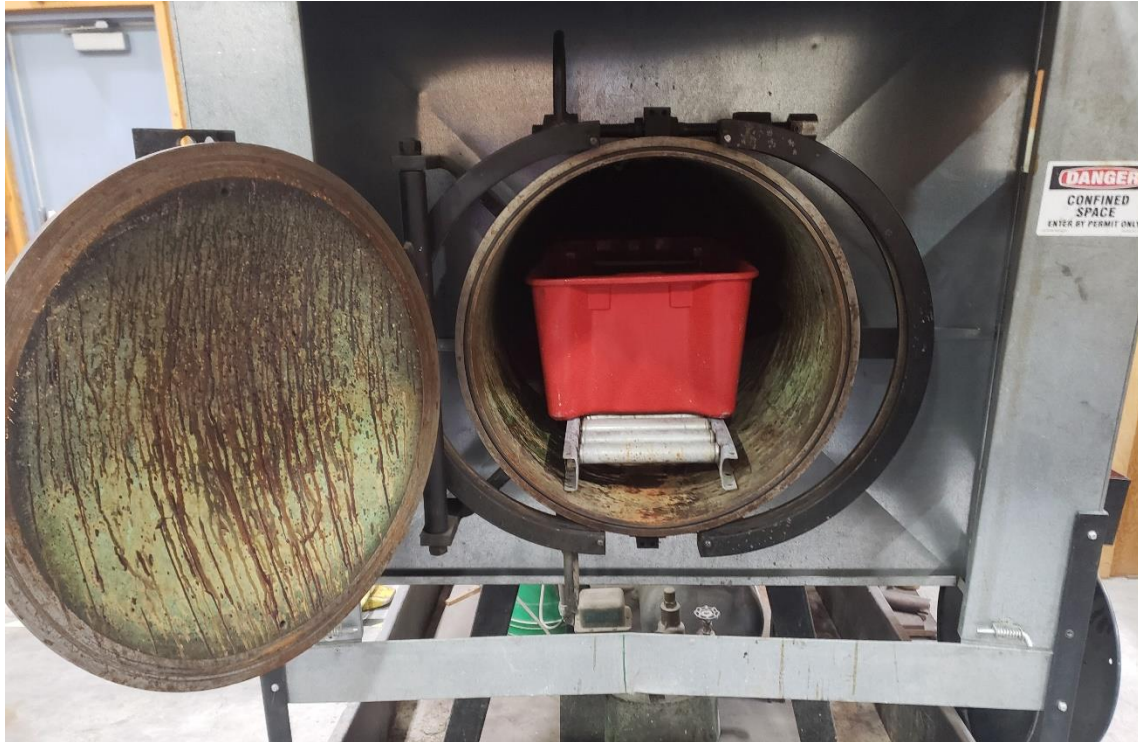
Figure 8. Cyclic delamination specimens within the ASCC pressure cylinder.
