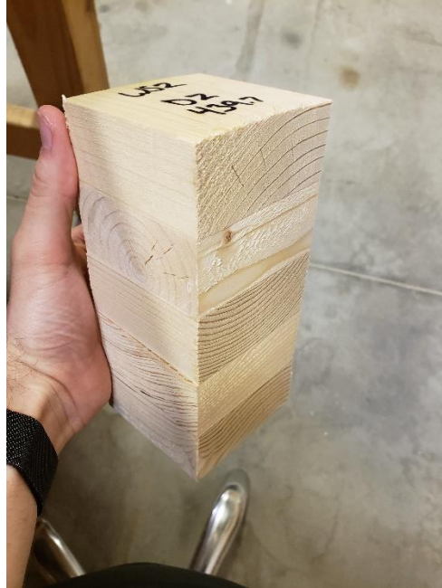
Figure 10. Example of Post Drying Delamination Sample
