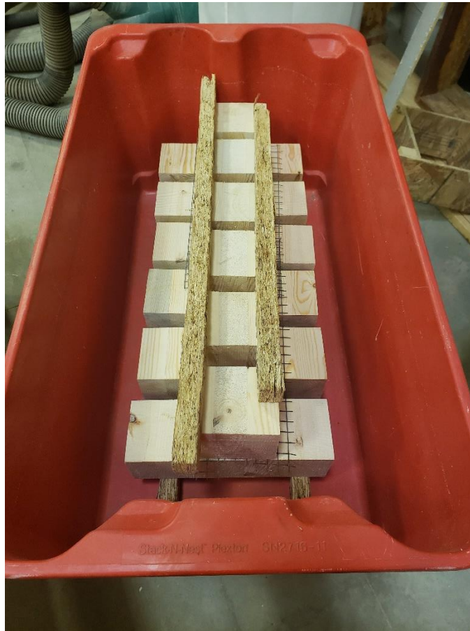
Figure 7. Cyclic delamination specimens being prepared for vacuum-pressure soak.
