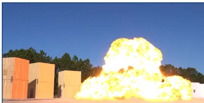
CLT Blast Testing at Tyndall Air Force Base
