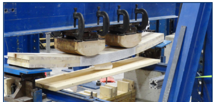
4-point Hybrid CLT Bending Test at UMaine
