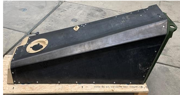
Figure 1 Carbon/PPS composite vehicle component fastened to vehicle end cap and pillar components, ready for assembly to vehicle.
