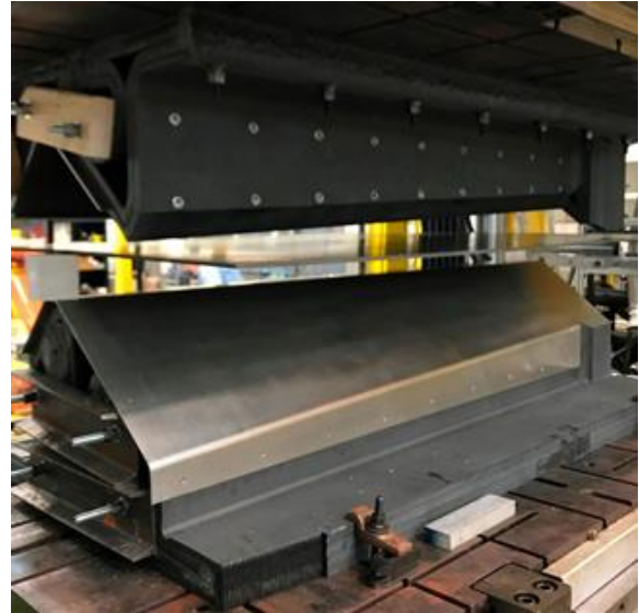
Figure 7 AM mold set in press. Sheet Metal cladding is clearly visible on the plug mold.
