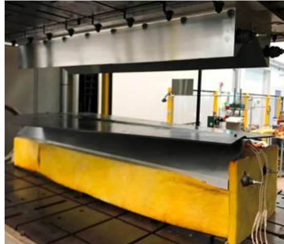
Figure 4 Fabricated metallic mold set. Plug mold is mounted to the press' bottom platen. Cavity mold is mounted to the press' upper platen.
