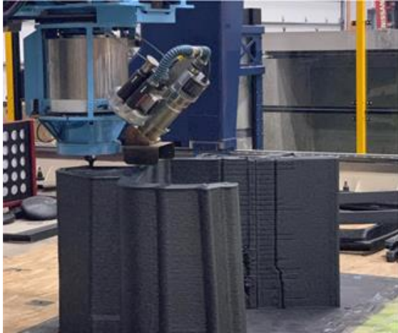
Figure 5 Two Large Scale AM molds being printed in one file then separated
