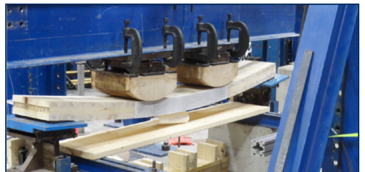
4-point Hybrid CLT Bending Test at UMaine
