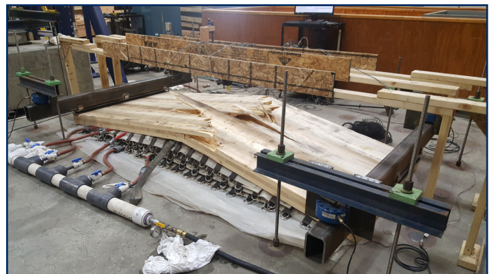
Uniform Load Bending Test of CLT at UMaine
