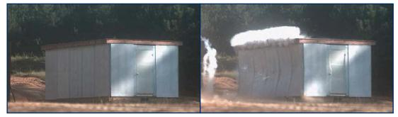
Left: Blast-resistant modular structure for force protection remained intact after 75' standoff blast.
