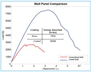
Uncoated wall panel fails in tension quickly, thus allowing little energy absorption. Coated wall panel assemblies show 2.4 times more strength and 4.4 times more energy absorption than uncoated panels.
