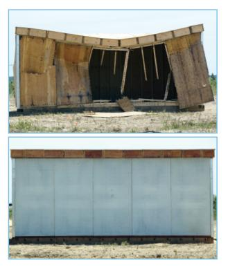
The images above show conventional construction (top) vs blast resistant construction (bottom) after truck bomb equivalent blast per UFC 4-0-10-01 DOD Antiterrorism Standards For Expeditionary Structures (Primary Gathering).
