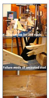
Failure mode of coated stud
