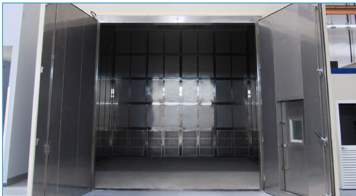
300 m 3 Three-story tall environmental test chamber
