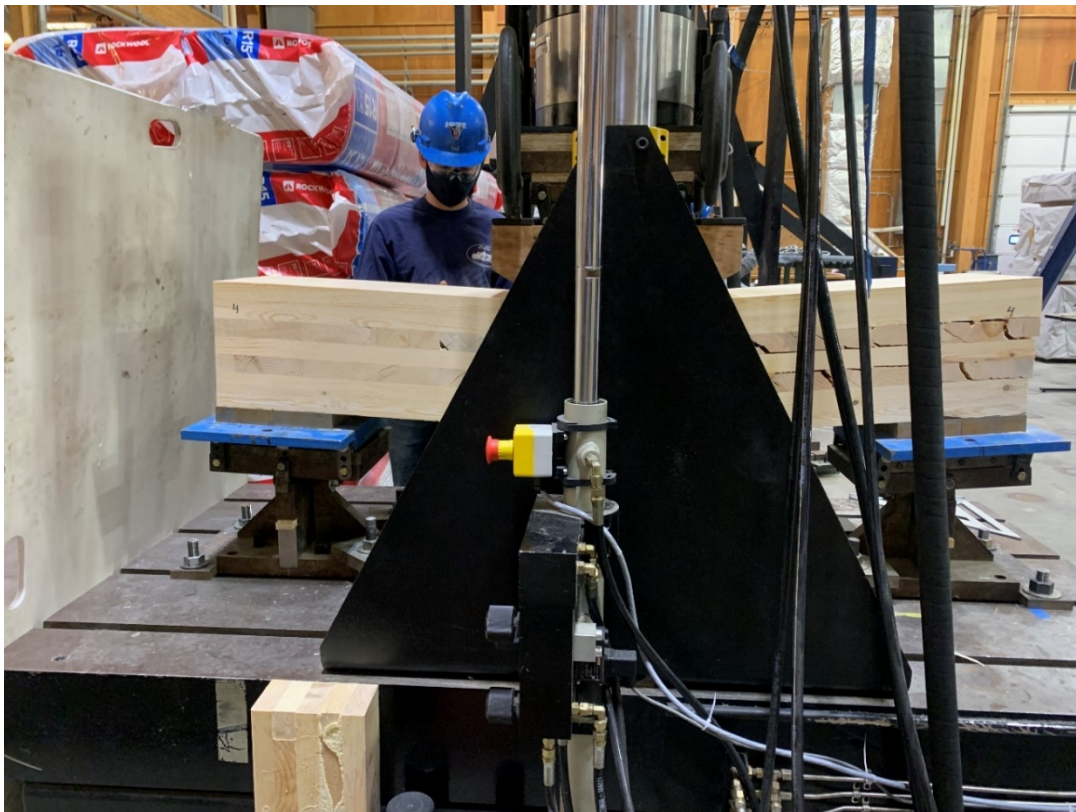
Figure 11. Flatwise shear modulus tests; 3-alt, minor strength direction (top) and 7-maxx, major strength direction (bottom).
