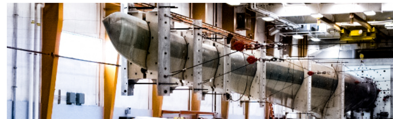
Flapwise testing of a 56 m wind blade.
