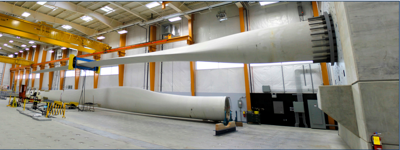
Wind blade fatigue testing with inertial resonance excitation
