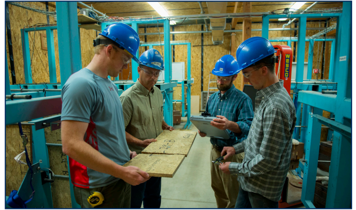
Testing is conducted according to ASTM D6815 - Standard Specification for Evaluation of Duration of Load and Creep Effects of Wood and Wood-Based Products.
