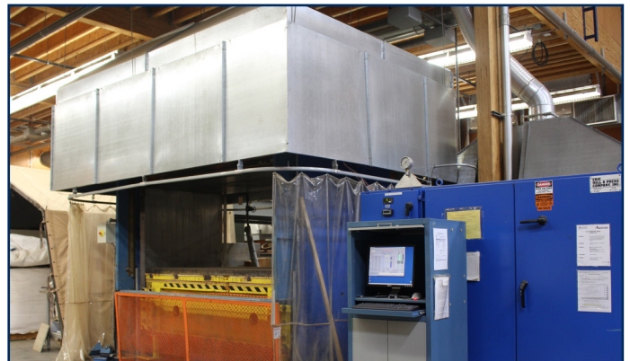
Top: 34" x 34" Dieffenbacher Steam Injection Press; Bottom: 4' x 8' Erie Mill & Press.
