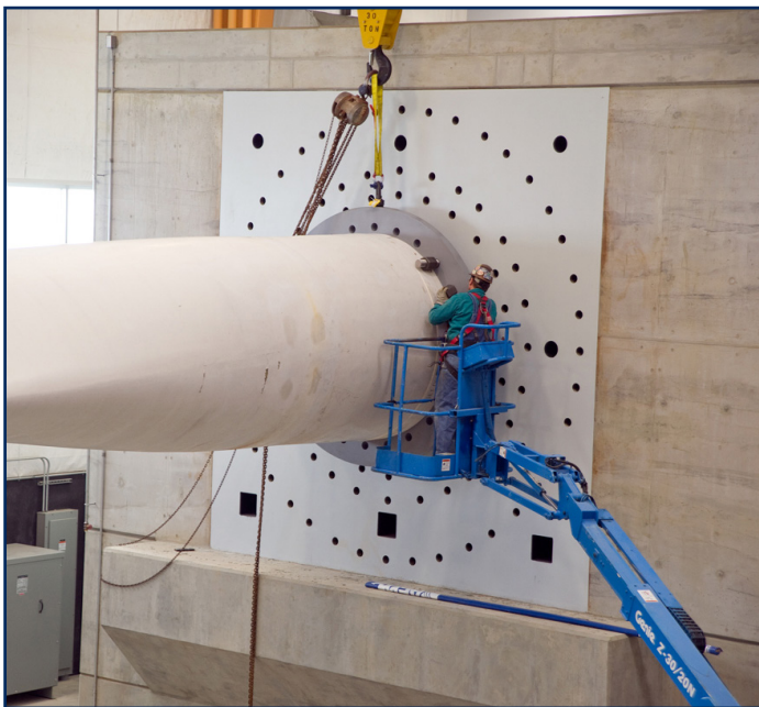
Offshore Wind Laboratory reaction wall
