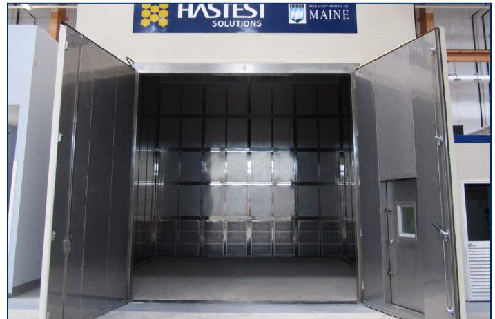
Offshore Wind Laboratory environmental test chamber
