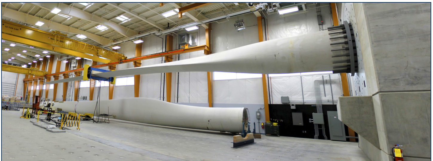
Wind blade fatigue testing with inertial resonance excitation
